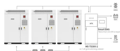
Application scenarios of energy storage battery products
